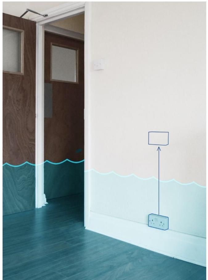
**Small changes and careful decisions can help make a house flood resilient and reduce cleanup after flooding. For example, choosing a kitchen with water resistant high gloss solid acrylic doors, or raising power sockets above the flood zone.**
